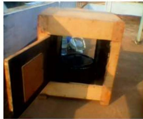
Figure 1 : Picture of the solar concentrator cooker      Figure 2 : Picture of box containing the pot
