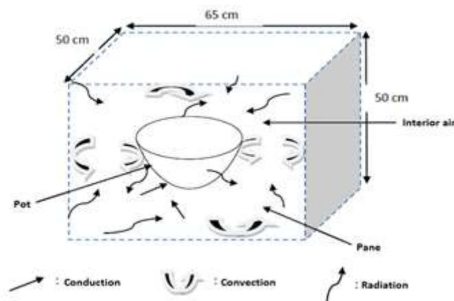
Figure 3 : synoptic scheme of the box solar cooker
