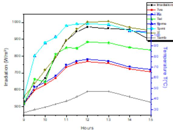
Figure 4 : Temperatures Profile of the parameters of the cooker with vacuum(24/10/2017)
