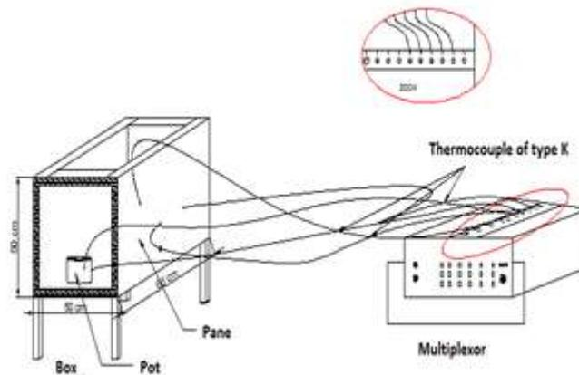
Figure 3 : Connexions between experimental device and data logger
